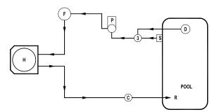
TYPICAL POOL - FLOW LESS THAN 70-GPM
