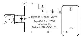
TYPICAL POOL - FLOW GREATER THAN 70-GPM
