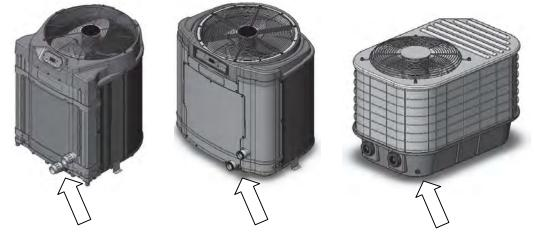
4. If no external drain plug is found, it will be necessary to open access panel and see if heat exchanger has an internal drain plug. If so, remove plug, and allow water to drain out of the condensor.
