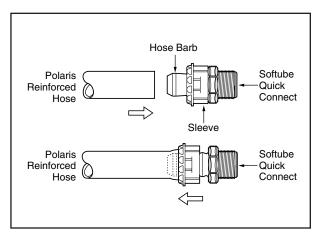
Warning: The Softube<sup>™</sup> quick connect is designed to work with the Polaris white reinforced hose (part #P19) only.
