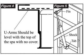
Step 5. Attach the enclosed BALL STUDS and LOCK NUTS to the TAB and the FIN located on the MAIN UNIT. Attach the SHOCK by pushing the female ends of each side over the BALL STUDS until they click into place. SEE FIGURE 5.
