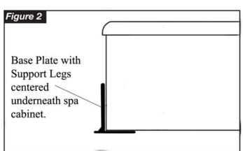
Step 2. Making sure that the spa is empty, slide the BASE PLATE underneath the center of the back of the spa cabinet. NOTE: This will be the side the spa cover will be stored behind. SEE FIGURE 2.
