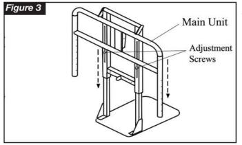
Step 4. Attach the Left and Right U-ARMS to the open tubes of the MAIN UNIT using the spring buttons (already attached.) Swing the U-ARMS up so they are parallel with the ground and using the ADJUSTMENT SCREWS, adjust the height of the MAIN UNIT so that the U-ARMS are level with the top of the spa without the cover. SEE FIGURE 4. NOTE: IF YOUR SPA COVER IS TOO THICK WHEN FOLDED TO FIT WITHIN THE U-ARMS, USE THE INCLUDED EXTENSION PIECE TO WIDEN THE ARMS.
