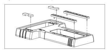
Figure 5. Snap Spacers into Place
