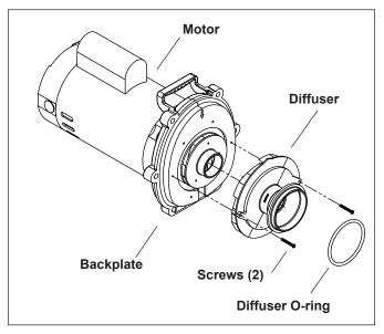
Figure 8. Remove the Diffuser
