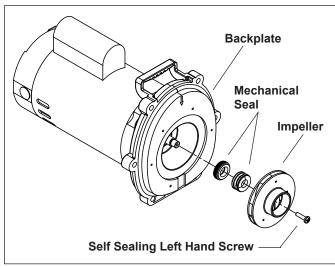
Figure 9. Remove the Impeller
