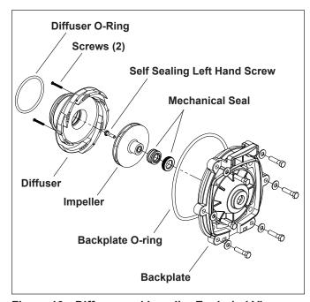
Figure 10. Diffuser and Impeller Exploded View
