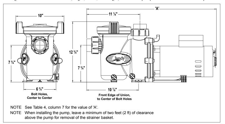
Figure 16. FHP Pump Dimensions (without Base or Spacers)
