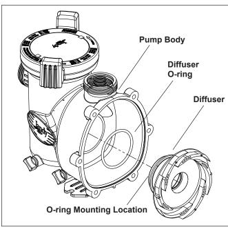
Figure 12. Pump Body and Diffuser Exploded View
