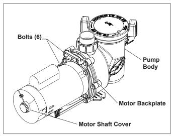
Figure 7. Remove the Pump Housing
