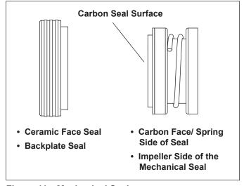
Figure 11. Mechanical Seal
