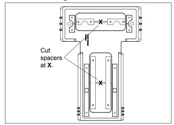
Figure 4. Cut Sets of Spacers Out of Base
