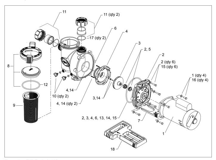
Figure 15. FHP Exploded View
